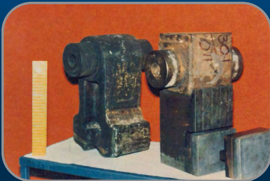
Before and after shots of two hammers. The left is manually hardfaced. The right is fitted with Vidaplate on the front and bottom faces to protect the shank while the bolt in Vidablock hammer does the crushing.
