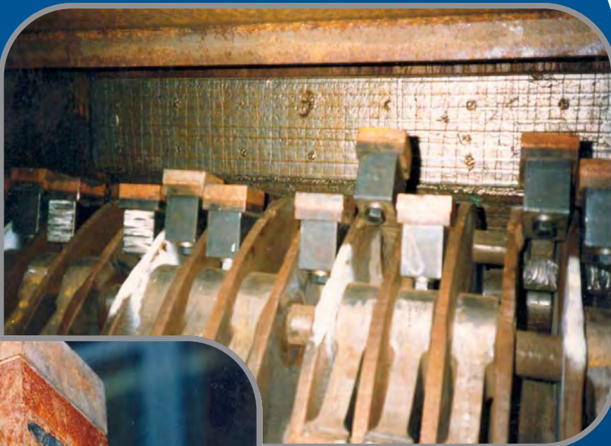
Inside of a cane shredder with Vidaplate hammer tips.
