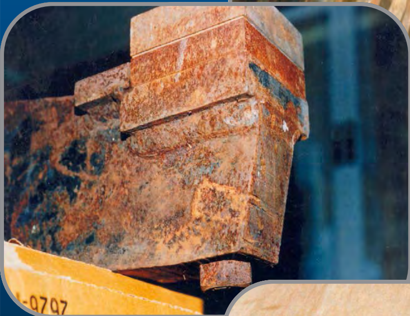
A sugar cane shredder hammer shank fitted with a 90mm x 90mm bolt on Vidablock.
