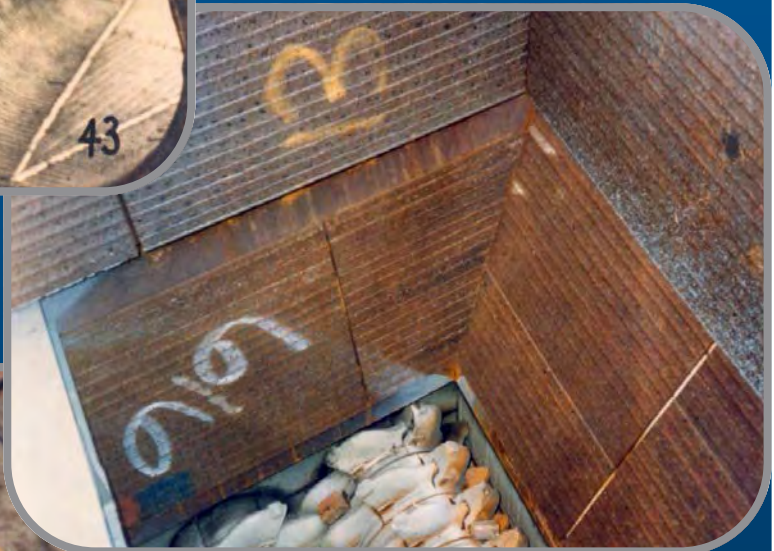
Stud attached liners on a rotary breaker feed chute.
