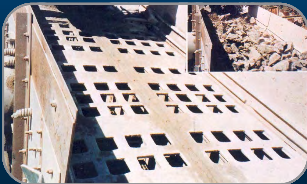
Vidaplate scalping screen fitted onto a screen deck.
