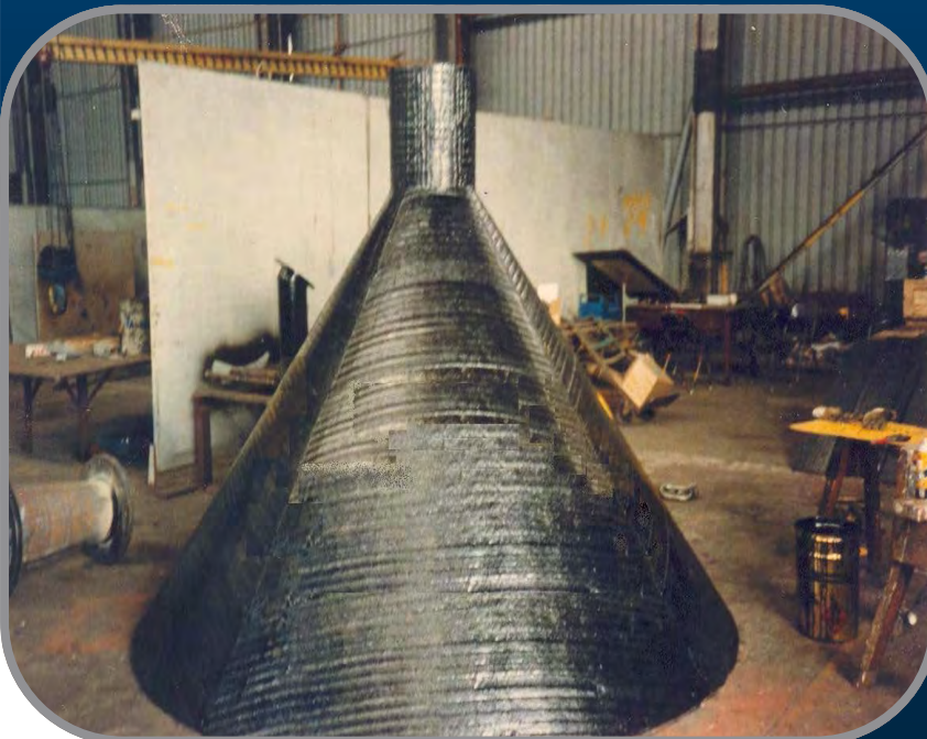
Cyclones fabricated for use in a cement manufacturing plant. The cones, cylindrical section, and inlet are all made from Vidaplate.
