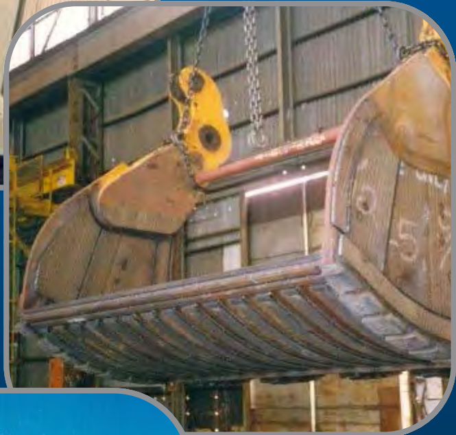
A Demag face shovel jaw fitted inside and out with Vidaplate.
