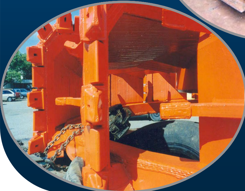
An example of Vidaplate on the bucket of a sand mining dredge.
