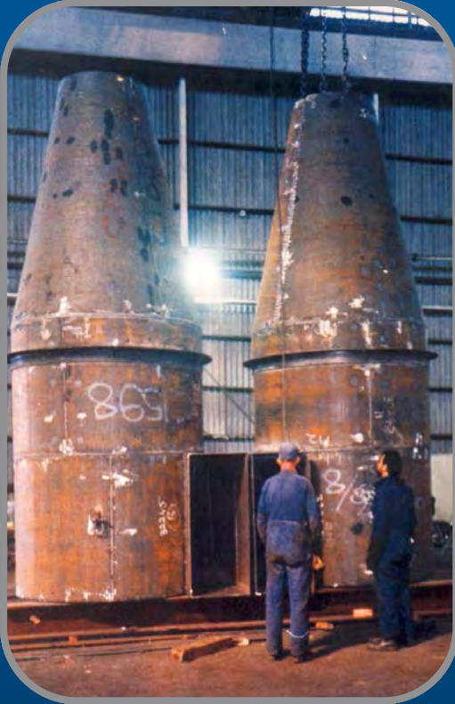
Cyclones fabricated for use in a cement manufacturing plant. The cones, cylindrical section, and inlet are all made from Vidaplate.
