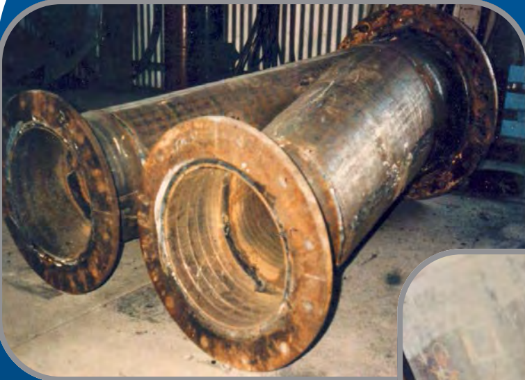
A fabricated Y section of pipe used in a copper smelter.
