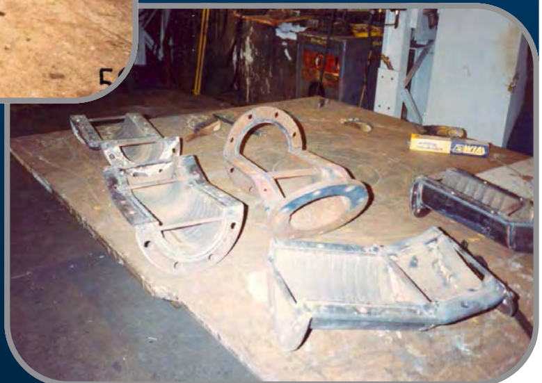
Fabricated replacement back sections that can be fitted to the back of a lobster back bend when it has worn away.
