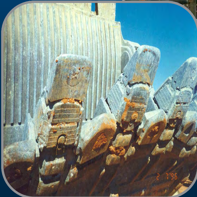
Vidaplate welded onto the adaptors.
