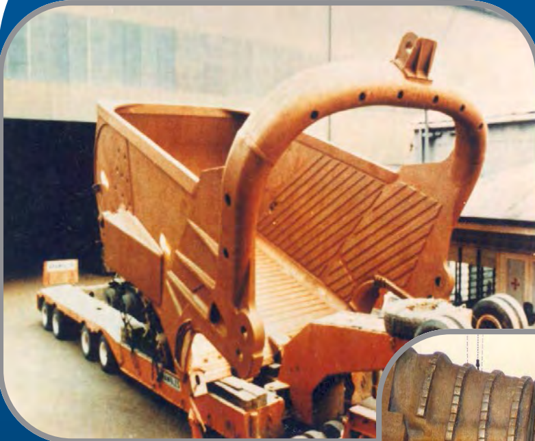
Dragline buckets lined with Bradken Vidaplate.
