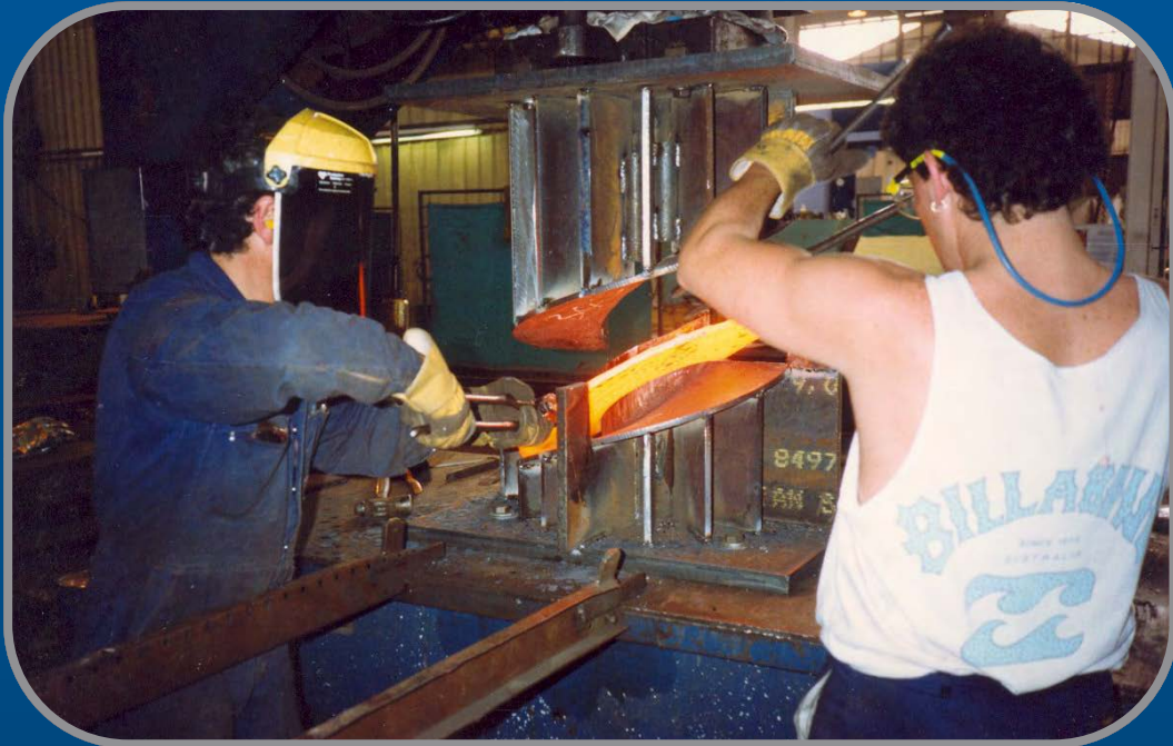
Heated flight section of a screw conveyor being placed into the male and female hot pressing die to have the helix and pitch pressed into it.
