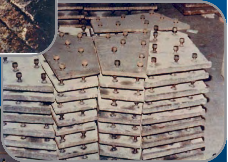
A set of Vidaplate liners showing the flash butt welded stud method of attachment.
