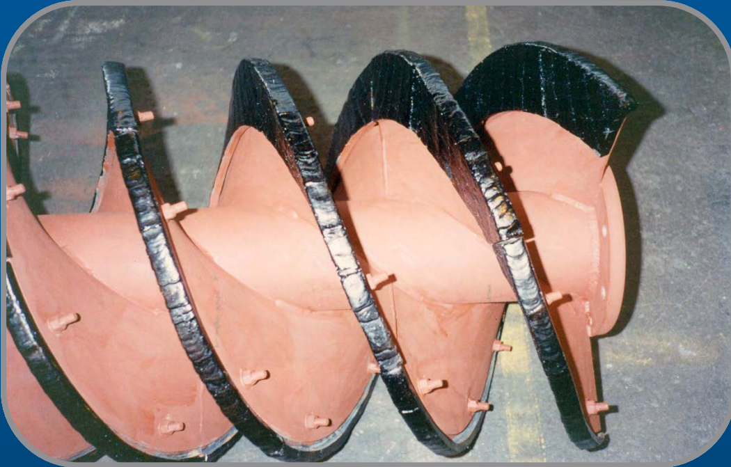
Replaceable bolt on screw conveyor flights
