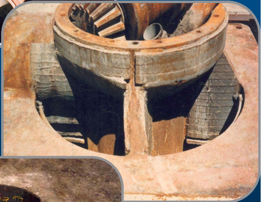
Manufactured protection ring and disc ready to be welded onto a Barmac impact crusher rotor. (See top picture)
