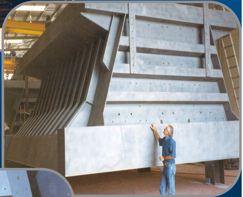
A large Vidaplate lined chute used in the iron ore industry.
