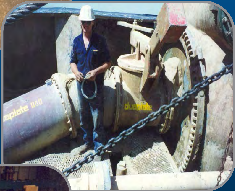
A straight pipe, elbow and T section fabricated from Vidaplate and fitted to a sand mining dredge.
