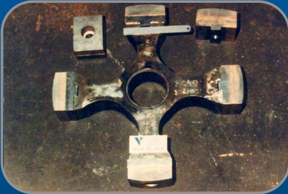
A four hammer rotor fitted with Duablock hammer tips that are positioned with a key and bolted into place.
