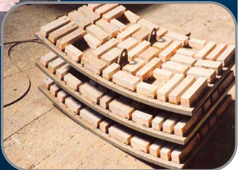
A range of different sized Vidablocks welded onto curved plates.
