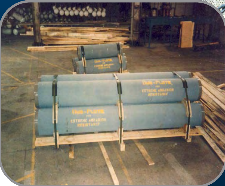
Straight pipe sections machined on the ends for Victaulic couplings.
