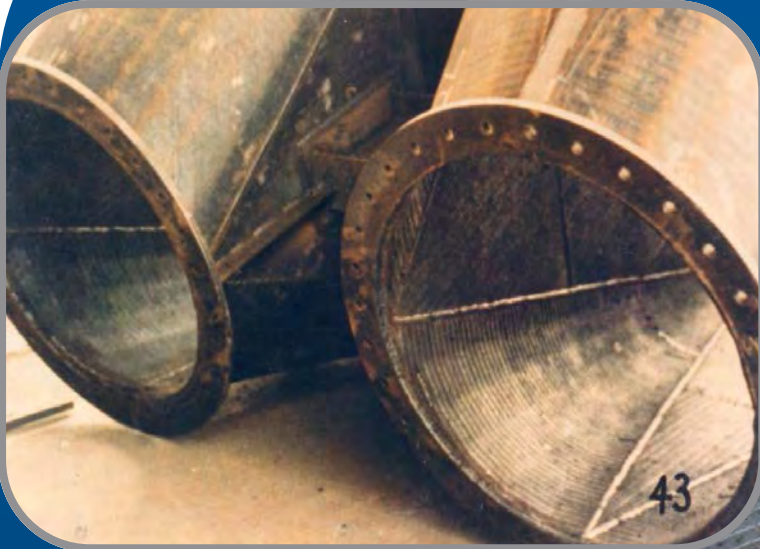
Stud attached liners on a rotary breaker feed chute.
