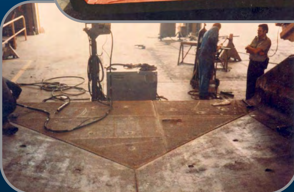
The lined dovetail area on a Cat 777 truck bed.
