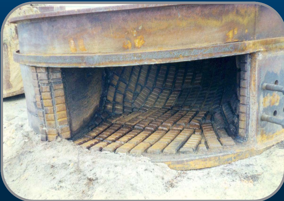
A dredge suction pipe bend lined with Choky block.
