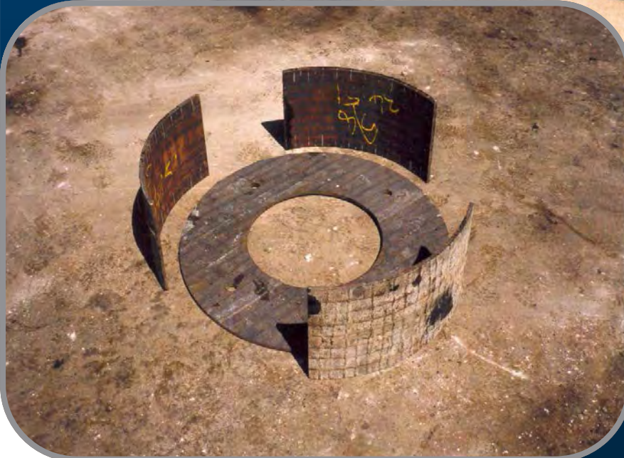
Manufactured protection ring and disc ready to be welded onto a Barmac impact crusher rotor. (See top picture)
