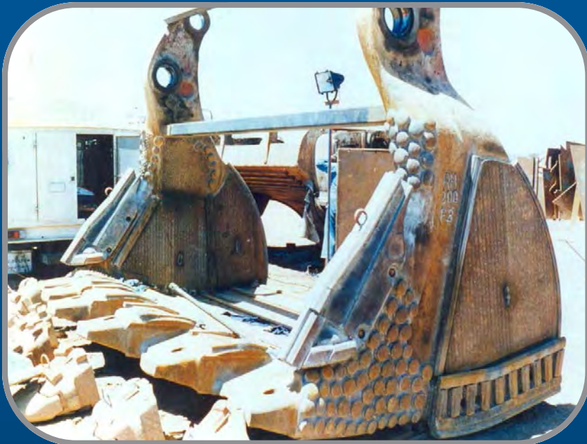
Face shovel buckets lined inside and out with Vidaplate and Vidabuttons.
