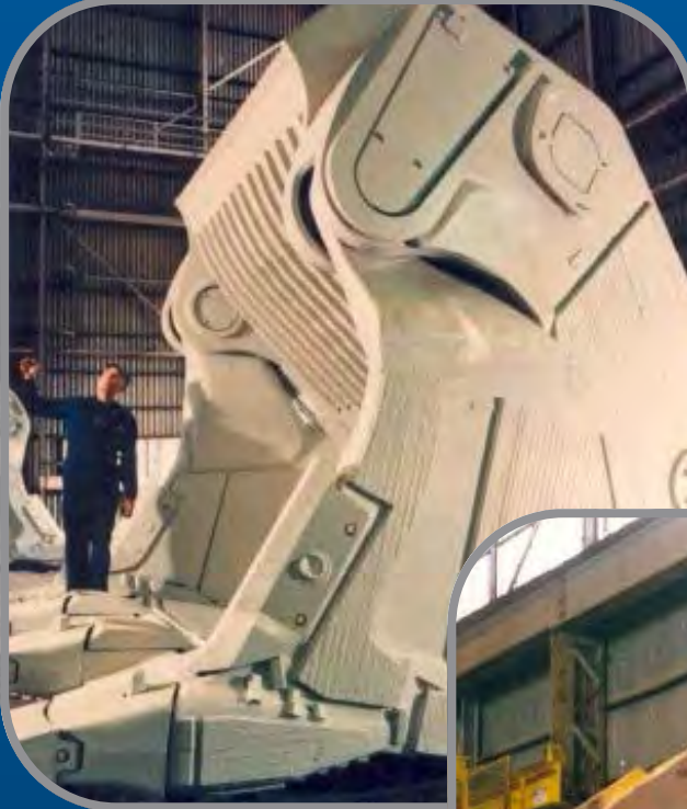
A Demag face shovel jaw fitted inside and out with Vidaplate.
