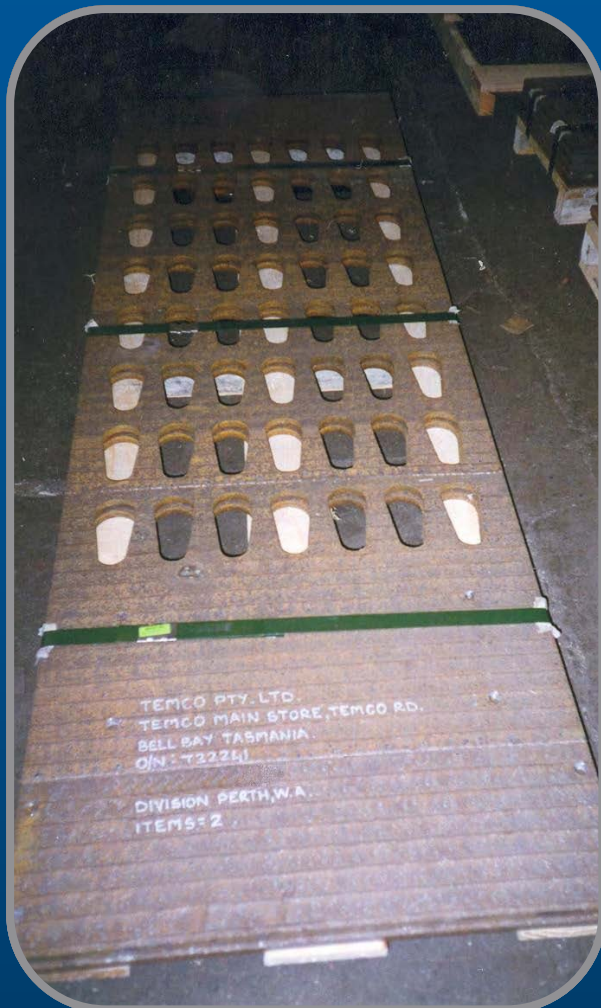
Teardrop shaped Vidaplate screen used in the production of Ferromanganese.
