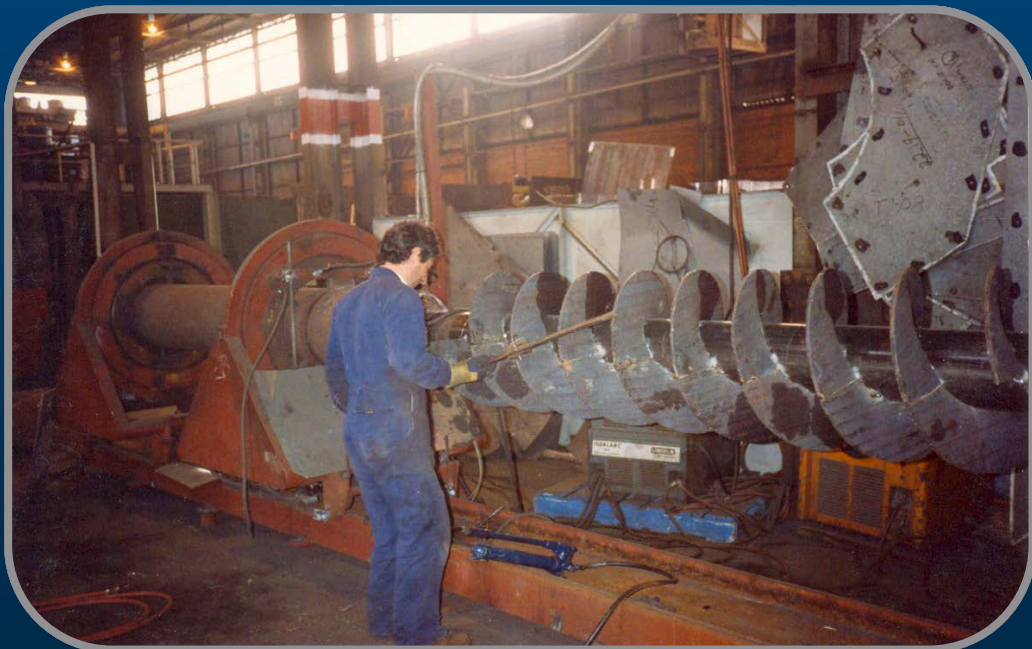
Flight sections are welded onto a tube section to complete the screw conveyor.
